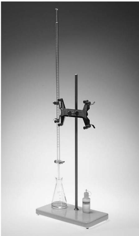
Typical setup for carrying out a titration
