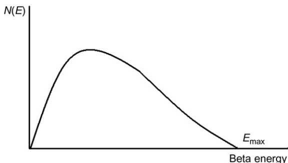
Figure 4.10 General shape of beta spectra: the number of beta particles with a given energy ( N(E) ) versus beta energy ( E ).
