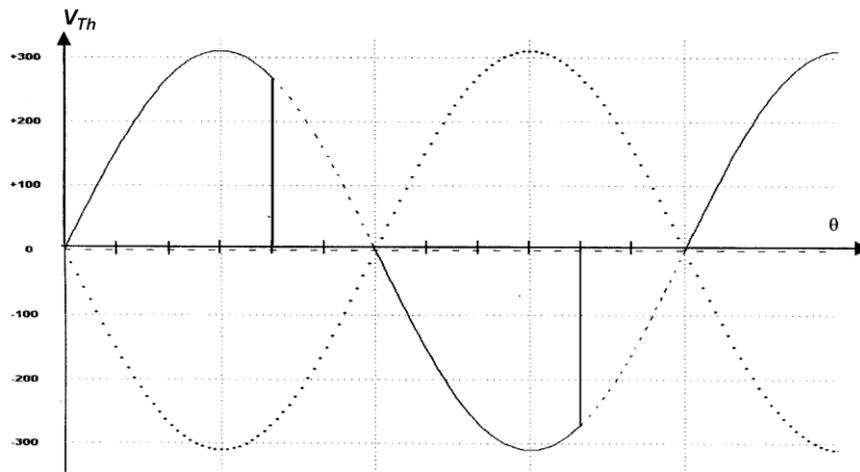
$$C_{12} \quad V_R^2 = \frac{\int_{\varphi}^{\pi} \hat{V}^2 \sin^2 \theta \, d\theta}{\pi}$$
