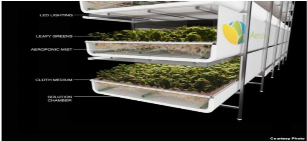
A diagram of an AeroFarms growing shelf. (Courtesy AeroFarms)
