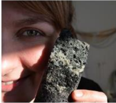
Geologist Sandra Shaebjornsdottir displays basalt encrusted with carbonate minerals formed from CO 2 . (© Kevin Krajick)
