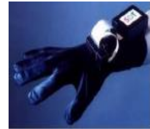
Digital glove (with position and direction sensors to interact with the virtual world in real time)
