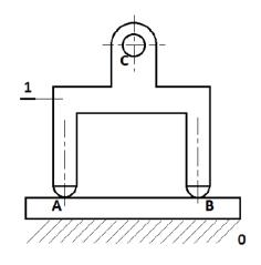
$\omega_{y} = \omega_{Ay}$   $\omega_{z} = \omega_{Az}$   $V_{x} = V_{Ax}$   $V_{y} = 0$
