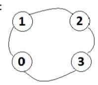
$$\vartheta_{0/0} = \vartheta_{0/1} + \, \vartheta_{1/2} + \vartheta_{2/3} + \vartheta_{3/0} = 0$$
