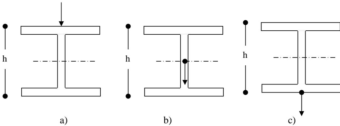
**Figure 2.** position de  $Z_g$  : a)  $Z_g = + h/2$ , b)  $Z_g = 0$  , c)  $Z_g = - h/2$
