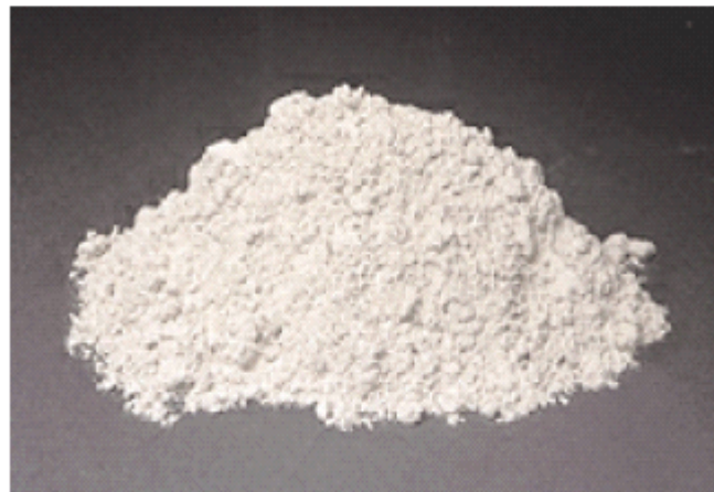
Fig. 3-5. Ground granulated blast-furnace slag. (69800)
