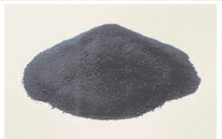
Fig. 3-7. Silica fume powder. (69801)
