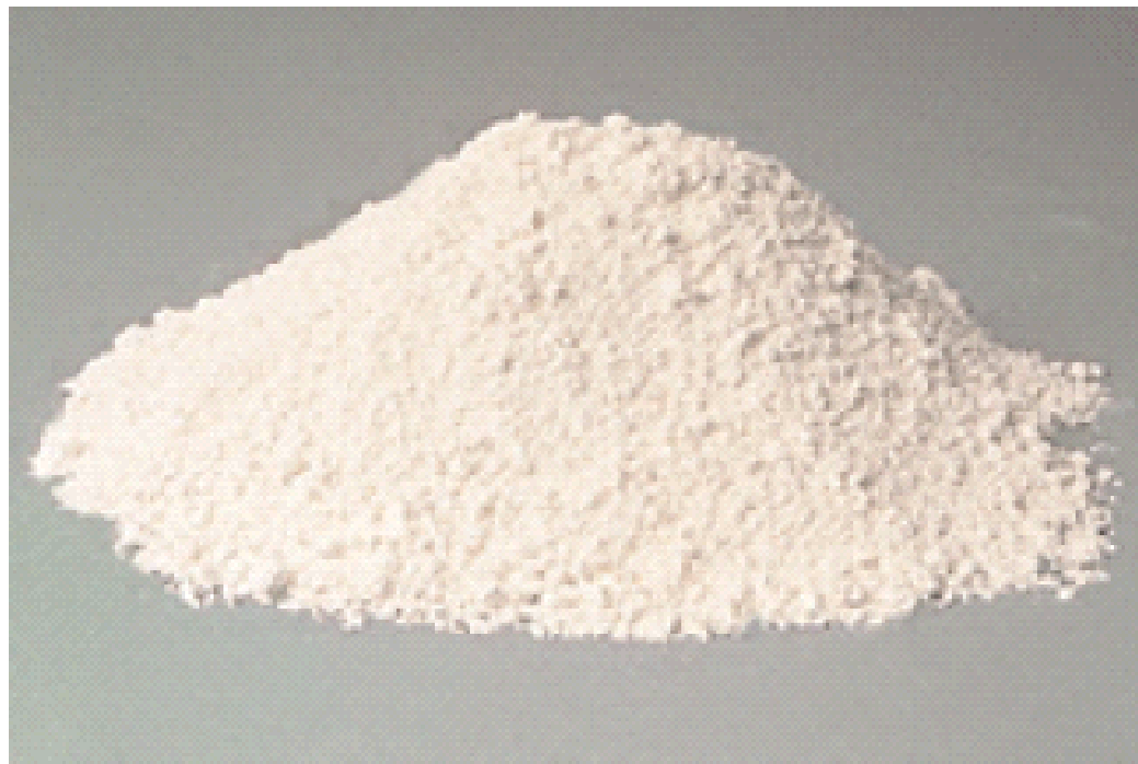
Fig. 3-11. Metakaolin, a calcined clay. (69803)
