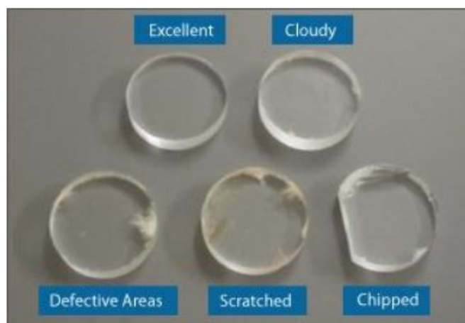
Fig.15: Sodium chloride (NaCl) plates in various conditions
