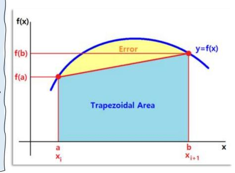
Truncation error estimation: Let's write and develop both I[f] and  $I_1[f]$ , using Taylor series
