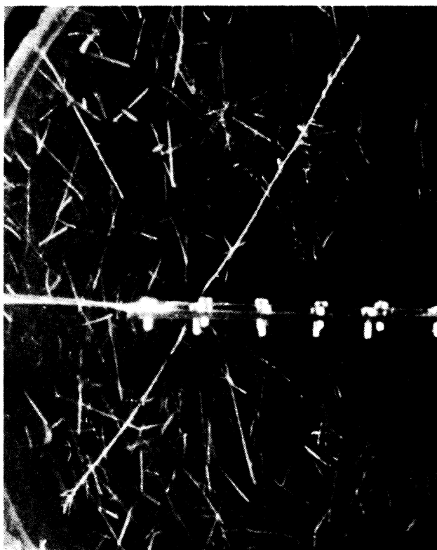
Fig. 9-14. Cloud-chamber photograph of the tracks of the two fragments resulting from the fission of a uranium nucleus [Bøggild, Brostrøm, and Lauritsen, Phys. Rev. 59 , 275 (1941)]. Initially the uranium nucleus was at rest in the thin horizontal metal plate at the center of the photograph. The two fragments move in opposite directions. From the analysis of the paths, we can estimate the energies of the fragments, which in turn (using the relation derived in Example 9.12) allow us to obtain the ratio of their masses. The effect of the neutrons released is neglected.
